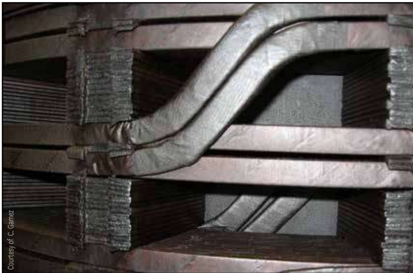
Figure 6: Example of transformer turns with degraded paper
