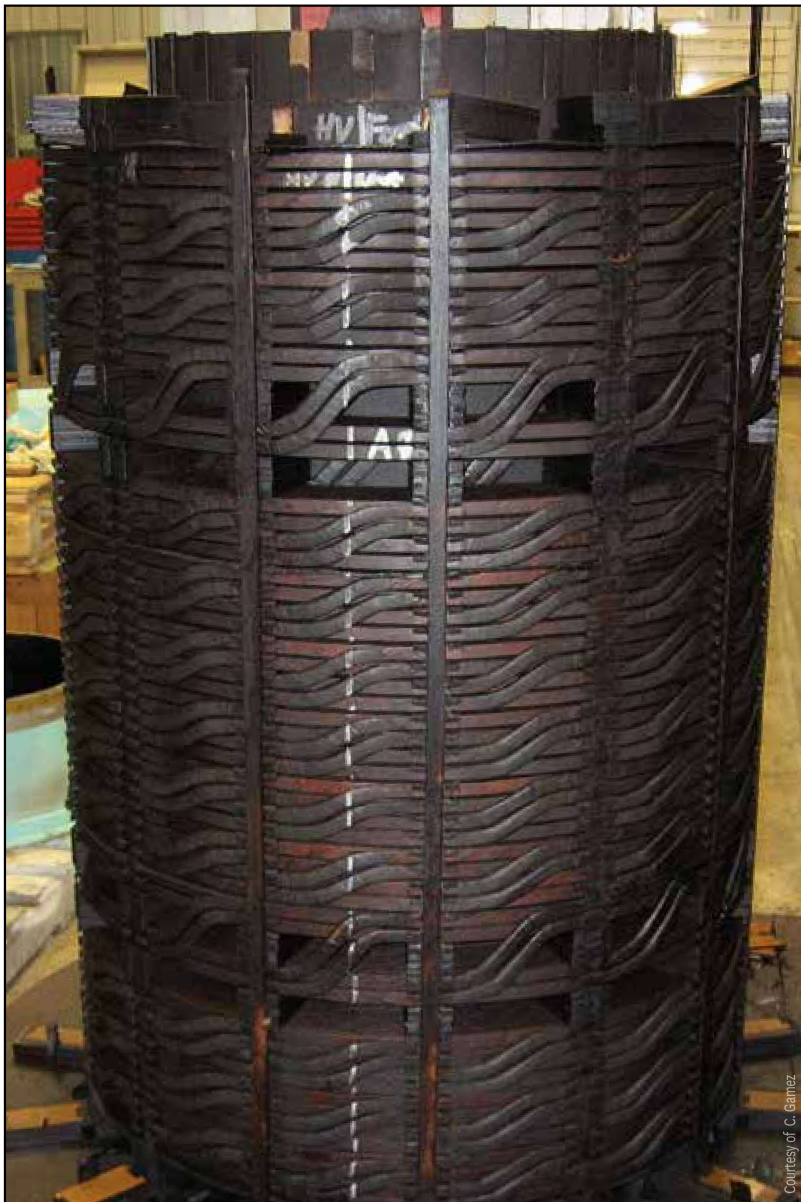
Figure 5: Example of transformer coil with degraded paper
