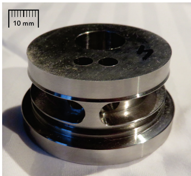
Figure 9 Base machined part of conformal cooling insert.
