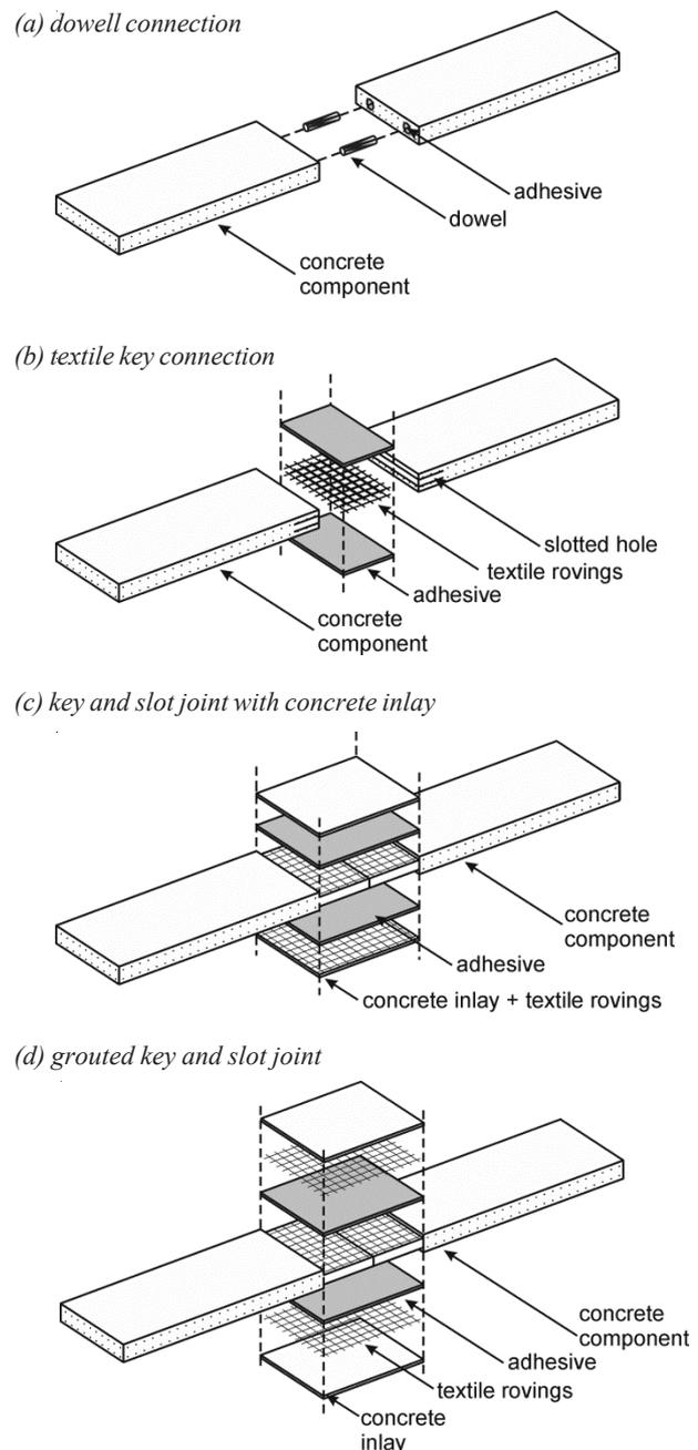
Fig. 2 Tested bonding technologies and geometries [11]
