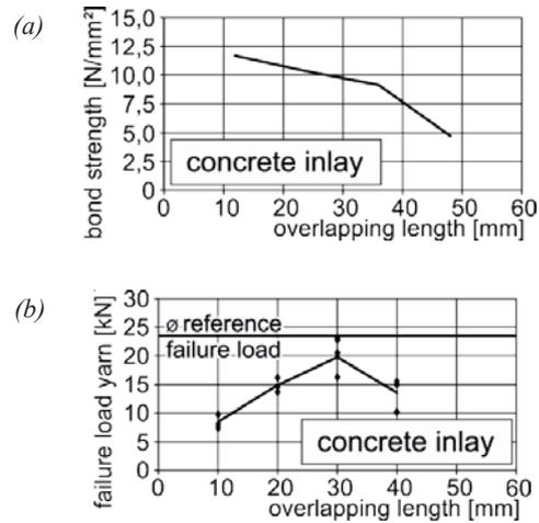
Fig. 18 Interdependence of bond strength (a) and failure load (b) with joint length (the tests on the key and slot specimens with a subsequently-grouted joint) [9]
