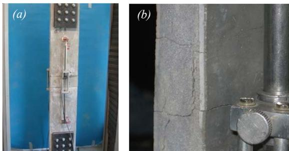
Fig. 9 Test set-up for the tensile tests (a); and concrete splitting under pure tension along reinforcement (b) [9]
