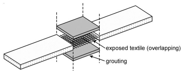
Fig. 21 Multiple layers of exposed, overlapping textile with subsequent grouting
