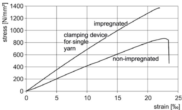
Fig. 4 Pull-out-tests: impregnated and unimpregnated rovings (2 x VET-RO-ARG-2400-01-05)
