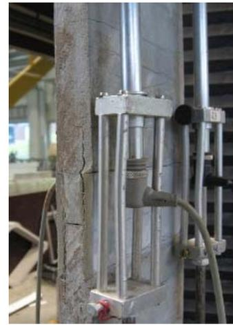
Fig. 12 Splitting cracks in the joint area of a key and slot specimen with a concrete inlay (a); subsequently grouted joint (b) [9]
