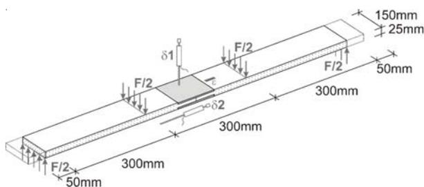
Fig. 15 Geometry of the specimens for the bending tests, configuration of the measuring devices [11]
