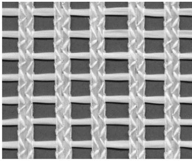
Fig. 3 Layout of textile rovings (source: Institut für Textiltechnik (ITA), RWTH Aachen University)
