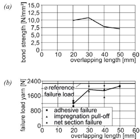
Fig. 5 Interdependence of bond strength (a) and failure load (b) with joint length (the bonded yarn tensile test)
