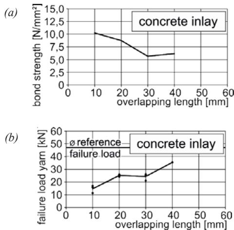
Fig. 11 Interdependence of bond strength (a); and failure load (b) and joint length (tests on the key and slot specimens with a concrete inlay) [9]
