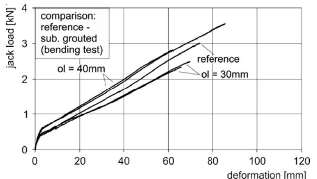
Fig. 19 Jack force – a displacement diagram of the selected subsequently-grouted key and slot specimens
