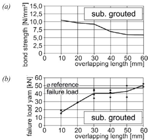
Fig. 14 Interdependence of bond strength (a) and failure load (b) with joint length (tests on the key and slot specimens with a subsequently grouted joint) [9]
