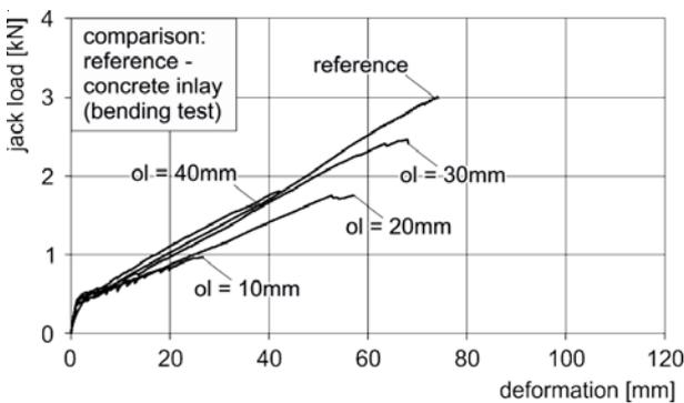
Fig. 17 Jack force – a displacement diagram of the selected key and slot specimens with a concrete inlay
