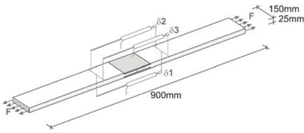
Fig. 8 Geometry of specimens for the tensile tests, configuration of measuring devices [11]
