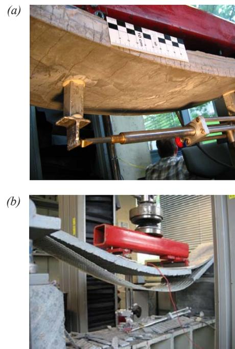
Fig. 16 Concrete cracking (a) and concrete spalling (b) during the bending test [9]
