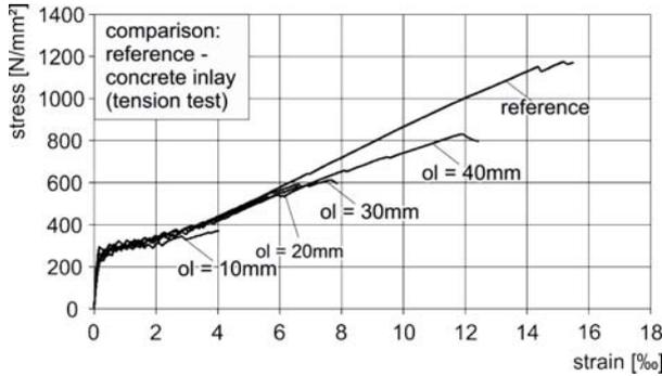
Fig. 10 Stress-strain behaviour of the selected key and slot specimens with a concrete inlay
