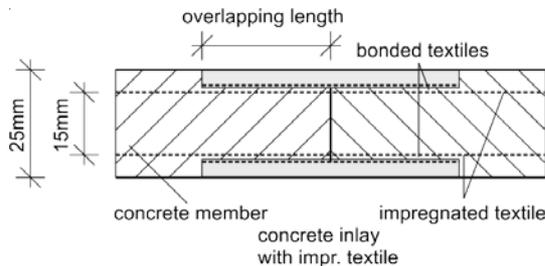
Fig. 6 Geometry of the key and slot joint with a concrete inlay
