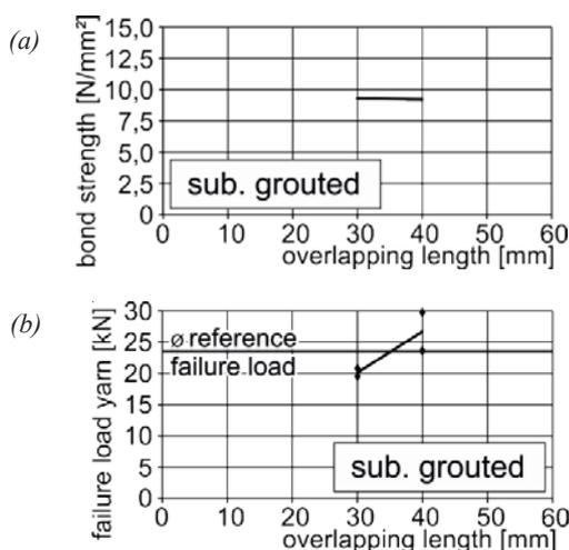
Fig. 20 Interdependence of bond strength (a) and failure load (b) with joint length (tests on the key and slot specimens with a subsequently-grouted joint) [9]
