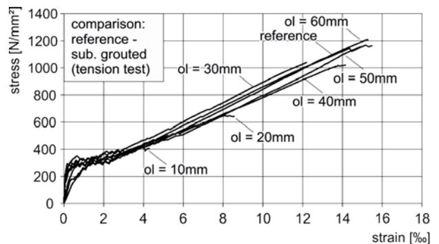
Fig. 13 Stress-strain behaviour of the selected key and slot specimens with a subsequently grouted joint
