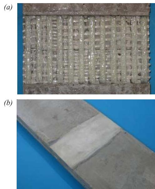
Fig. 7 Bonded textile straps (a); and the final key and slot concrete member with subsequent grouting (b)
