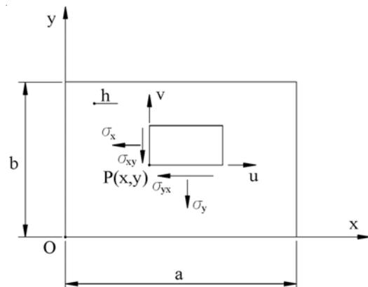
Fig. 1 Rectangular plate for in-plane vibrations
