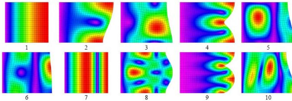
Fig. 5 Natural modes of in-plane vibrations of a rectangular plate,  $a/b=1.2$ , C-SS2-F-SS2
