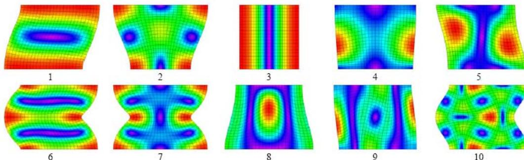
Fig. 4 Natural modes of in-plane vibrations of a rectangular plate,  $a/b=1.2$ , F-SS2-F-SS2
