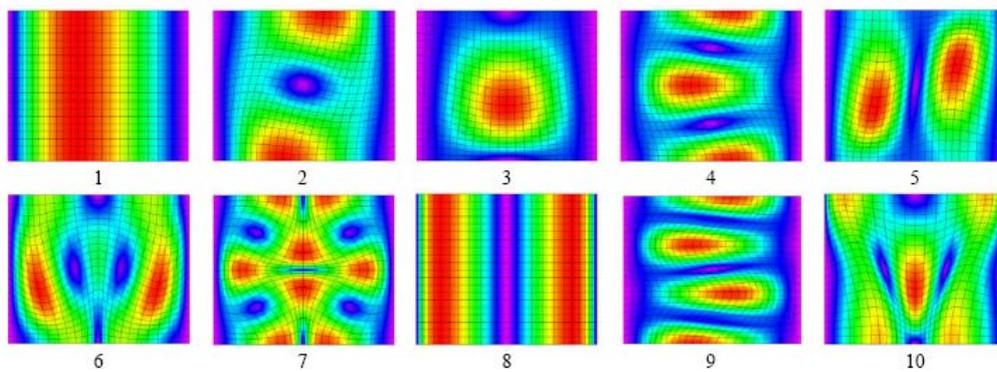
Fig. 3 Natural modes of in-plane vibrations of a rectangular plate,  $a/b=1.2$ , C-SS2-C-SS2
