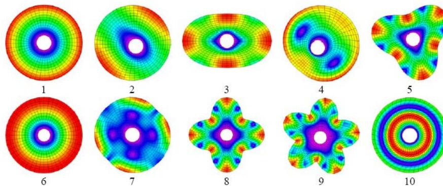
Fig. 8 Natural modes of a clamped-free annular plate,  $r_0/R=0.2$
