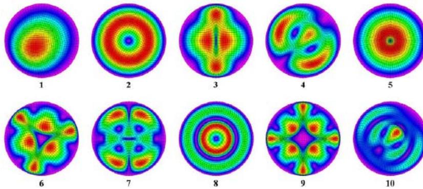
Fig. 6 Natural modes of a clamped circular plate
