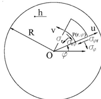
Fig. 2 Circular plate for in-plane vibrations
