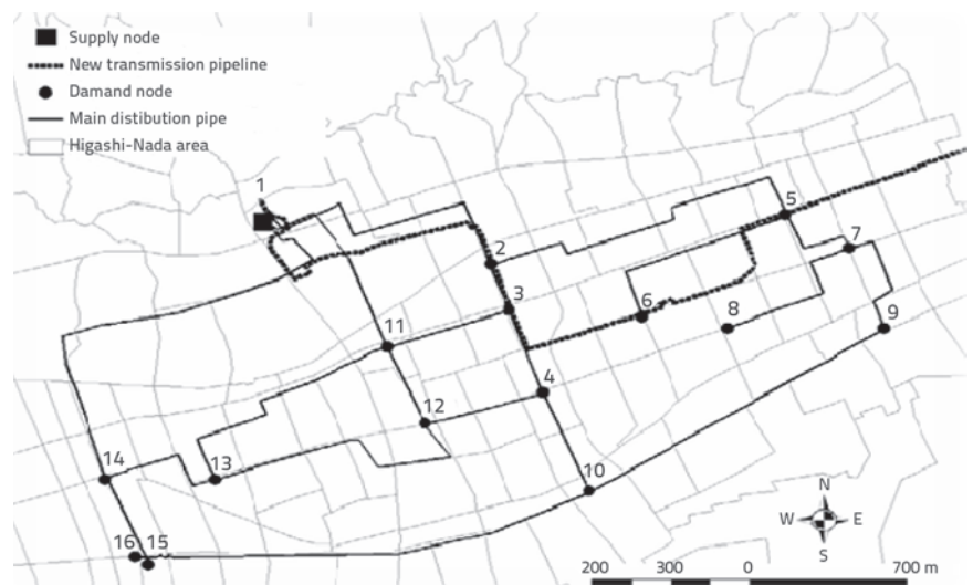
Figure 14. Main water distribution pipeline in Higashi-Nada ward of Kobe city [12]
