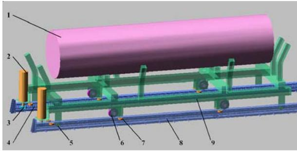
Legend: 1. DSRV; 2. Motor; 3. Drive gear; 4. Rack; 5. Reverse-wheel; 6. Load-bearing wheel; 7. Horizontal wheel; 8. Track; 9. Vehicle body
