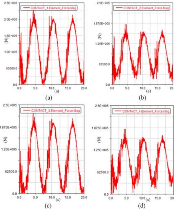
Fig. 7 Contact forces of the load-bearing wheels
