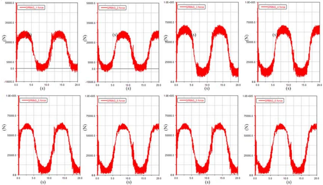
Fig. 11 Tensile forces of 8 lashing bars
