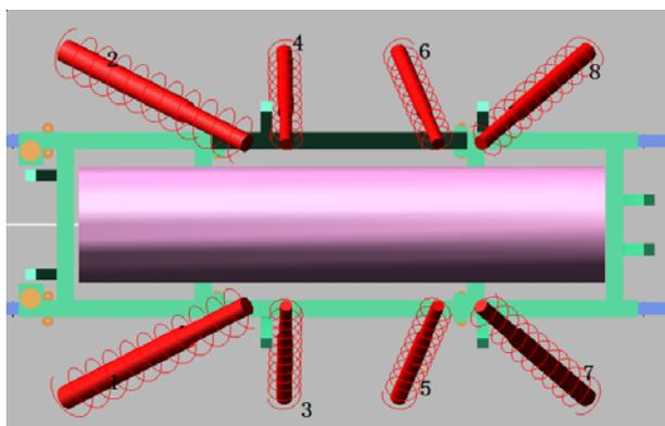
Fig. 4 Dynamics model of LV-DSRV with lashing bars
