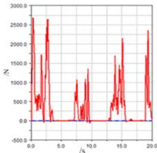
Fig. 12 Comparison of contact forces for cases of 1 mm gap and no gap
