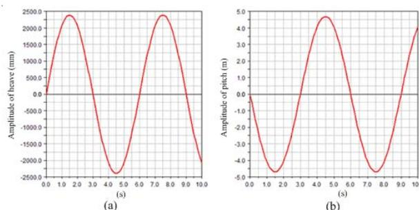
Fig. 5 Ship motion in heave (a) and pitch (b) at the sea state 5
