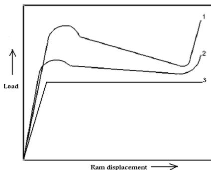
Fig. 2 Load vs. displacement curves for forward (curve 1) & backward (curve 2) conventional extrusion and open die extrusion (curve 3)
