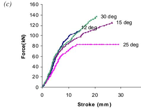
Fig. 9 Force – Stroke diagram for open die extrusion at (a) 0.09 strain, (b) 0.13 strain and (c) 0.21 strain
