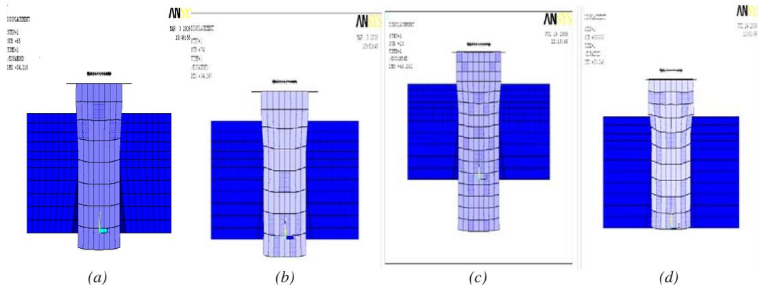
Fig. 4 The grid deformations at extrusion strain of 0.09 for die angles of (a) 12°, (b) 15°, (c) 25° and (d) 30°
