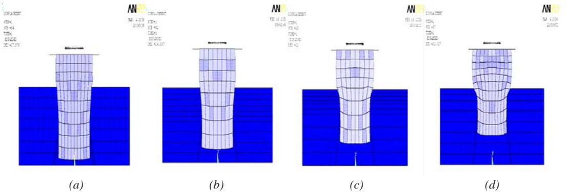
Fig. 5 The grid deformations at extrusion strain of 0.13 for die angles of (a) 12°, (b) 15°, (c) 25° and (d) 30°
