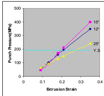
Fig. 10 Variation of experimental punch pressure with extrusion strain
