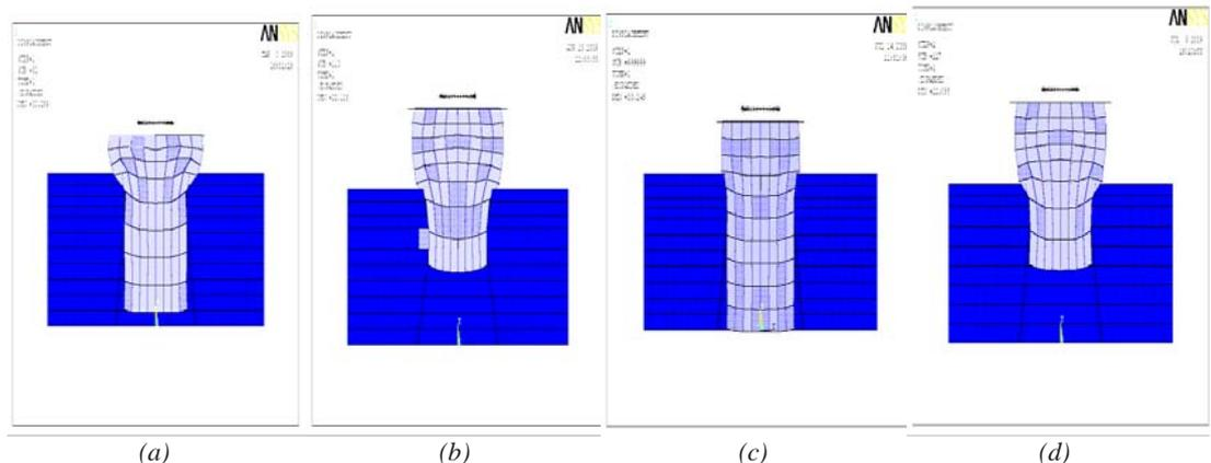
Fig. 7 The grid deformations at extrusion strain of 0.21 for die angles of (a) 12°, (b) 15°, (c) 25° and (d) 30°
