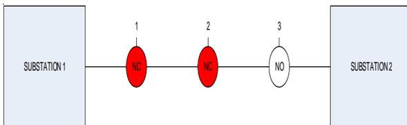
Fig. 4 Operating condition in case of a fault between point 3 and substation 2
