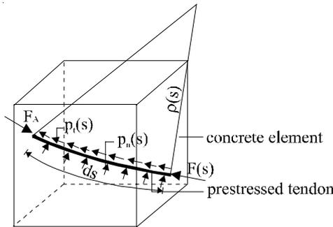
Fig. 4 Concrete finite element with embedded prestressed tendon finite element
