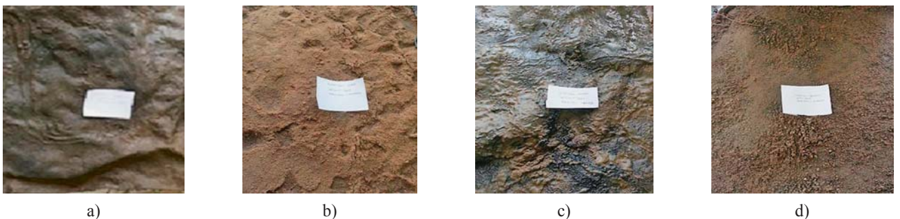
Fig.3 Jute geotextile samples removed from different road designs subjected to 100 mm/hr rainfall intensity: a) 60 days without sand layer, b) 60 days with sand layer, c) 90 days without sand layer, d) 90 days with sand layer
