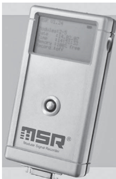
Fig.3 Modular measuring system MSR 12 for measuring physiological parameters of human body in accordance with standard ISO 9886:2004 [22]
