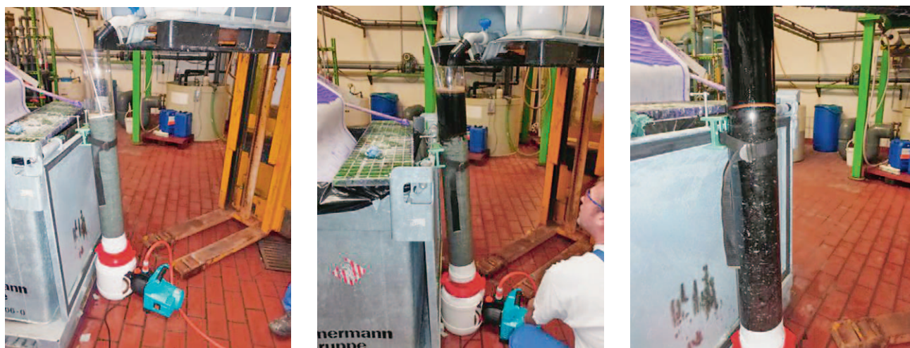
Fig.8 Operational on-road test for the recovery of palladium from industrial process waters by the use of PVAm-modified PET textiles
