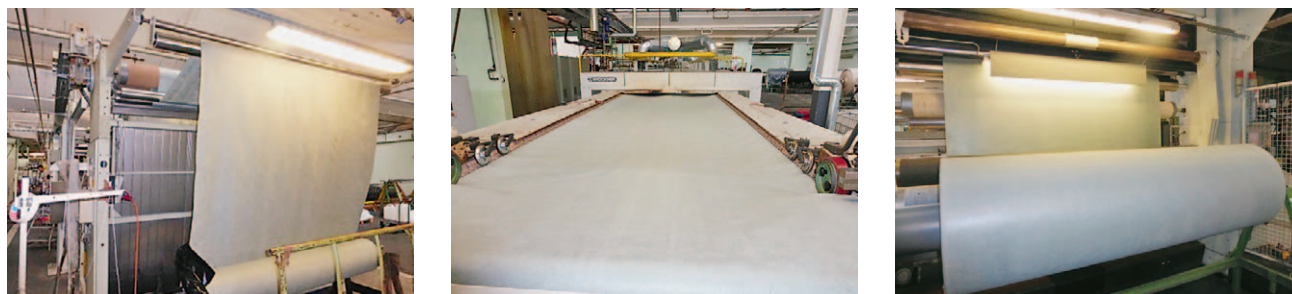
Fig.6 Finishing of polyester with polyvinylamine on industrial level
