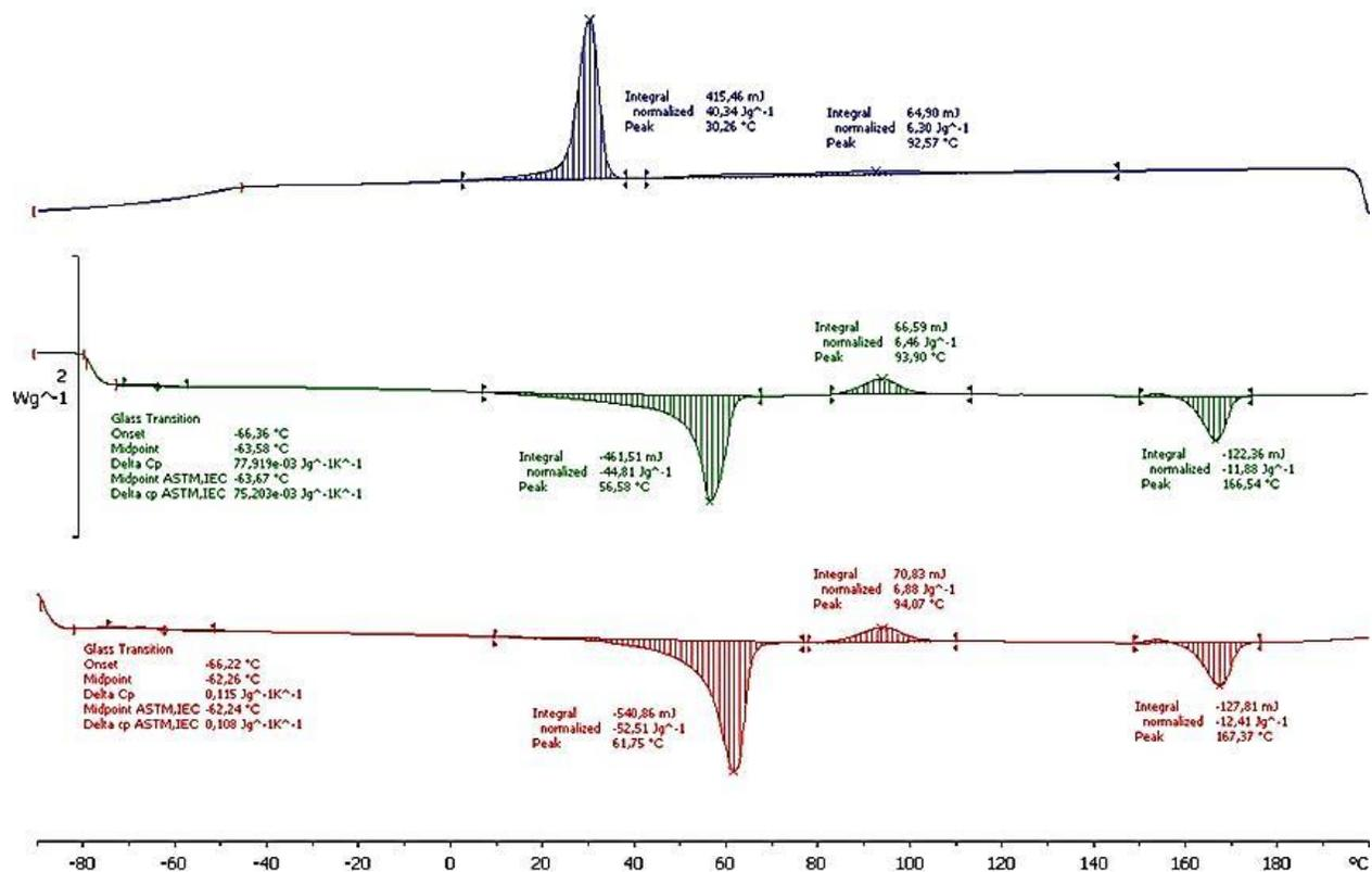
Figure 4 DSC thermograms of 1<sup>st</sup> and 2<sup>nd</sup> heating cycles and cooling cycle for sample PCL/PLA 70 %/30 % + 3 % of fibres
