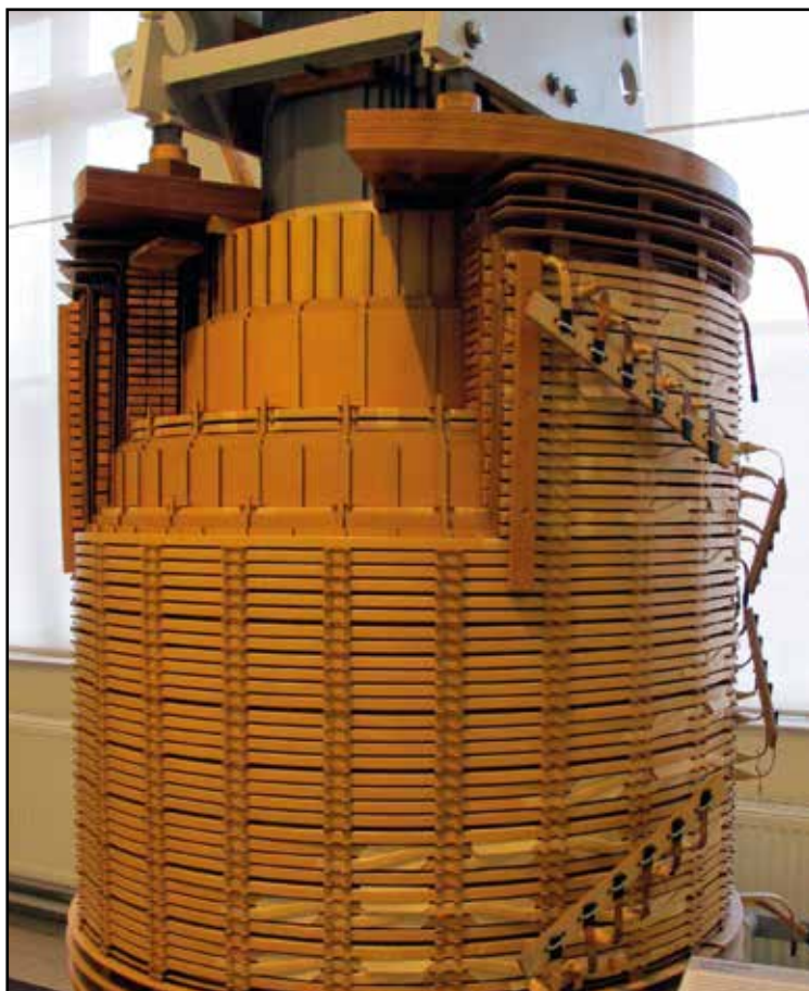
Figure 2: Insulation in power transformer
