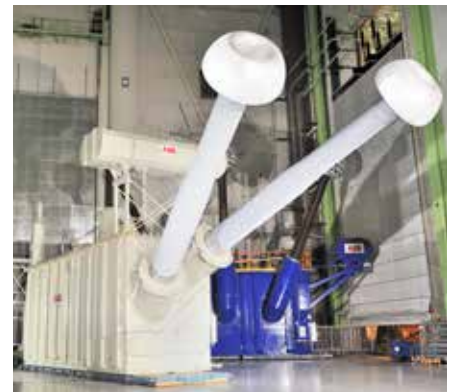
Figure 7: HVDC converter transformer [4]
