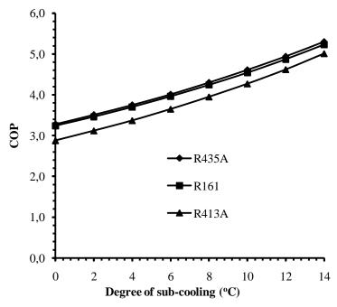
**Figure 8.** Variation of coefficient of performance (COP) with the degree of sub-cooling at 40  $^{\circ}$ C condensing and -20  $^{\circ}$ C evaporating temperatures
