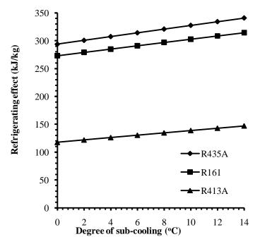
**Figure 6.** Variation of refrigerating effect with the degree of sub-cooling at 40  $^{\circ}$ C condensing and -20  $^{\circ}$ C evaporating temperatures
