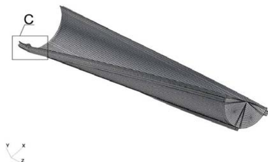
Fig. 23 Version 1- riveted joint of the skin with the stringer, local post buckling deformation
