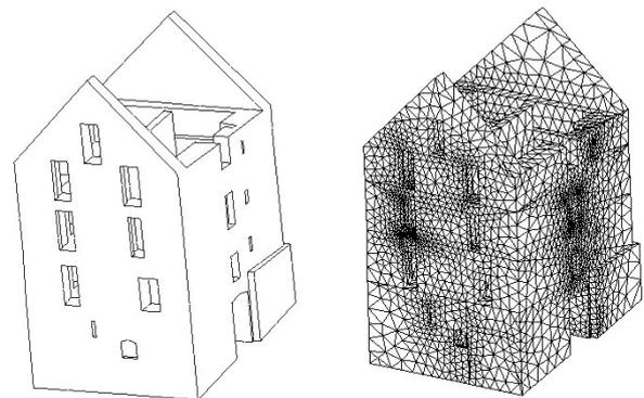
Fig. 9 P – model: geometry and mesh idealisation
