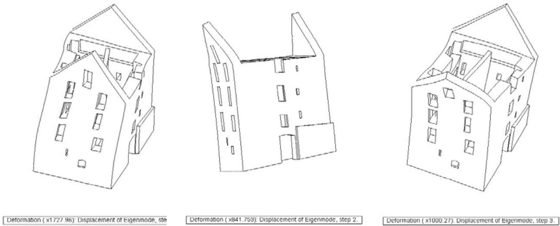
Fig. 11 1<sup>st</sup>, 2<sup>nd</sup> and 3<sup>rd</sup> modal shape for model PS
