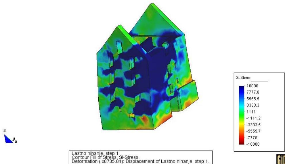
Fig. 12 PS1 model: Seismic analysis for the 1<sup>st</sup> modal shape – results for main tensile stresses
