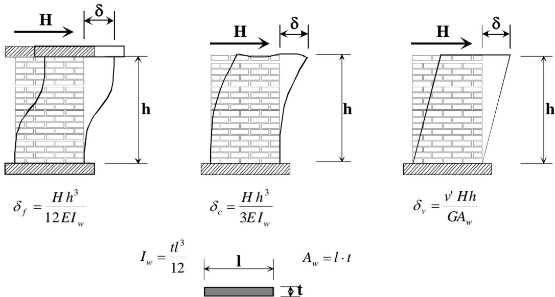
Fig. 1. Elastic deflections of masonry walls
