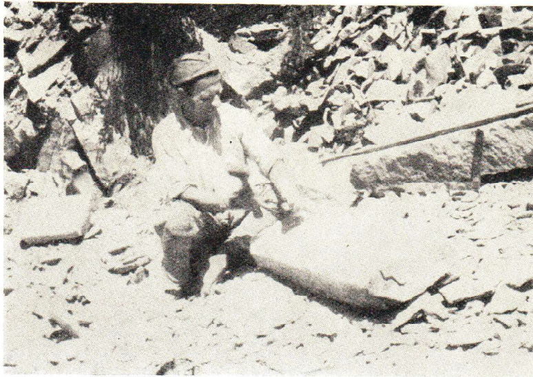
Fig. 6. Final dressing of stone is often done right in the quarry. The stonecutter wears no protective goggles, he is bare-footed and unprotected from sun Sl. 6. U kamenolomu »Pešćar« često se vrši i definitivna obrada tamo izvadene stijene. Kamenorezac nema nikakvih zaštitnih naočari, on je bos i nije zaklonjen od sunca
