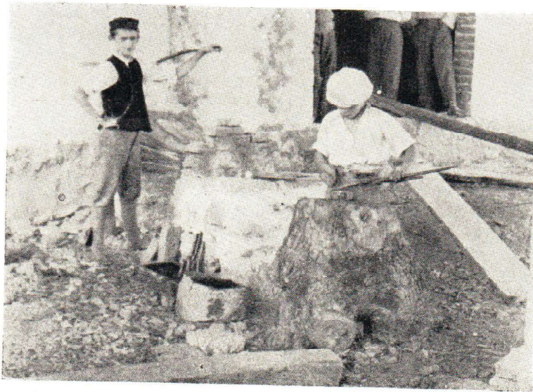
Fig. 3. Even the youngest stonecutters are good as forging and welding. One boy on the left blows the bellows while the one on the right makes a »špic« (sort of small pick and hammer without shaft, combined in one tool, cf. »m« on Fig. 12) on an anvil of heated iron
