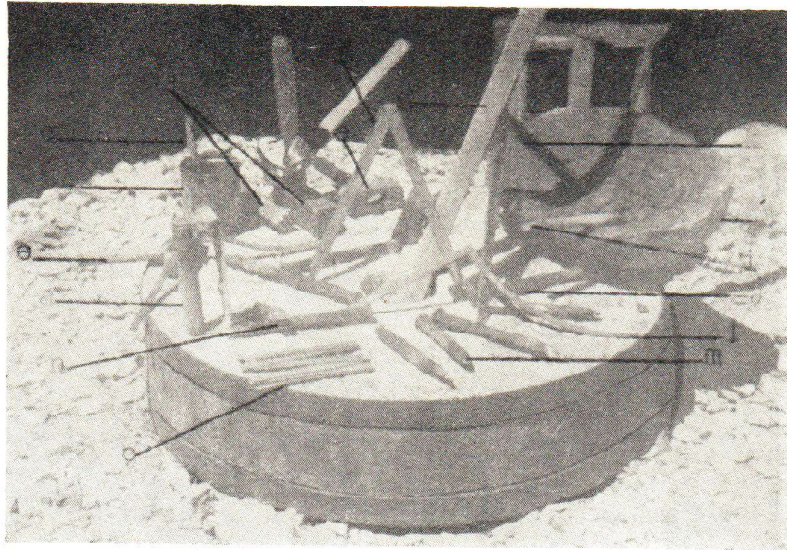
Fig. 12. Stonecutters' tools in use to-day
