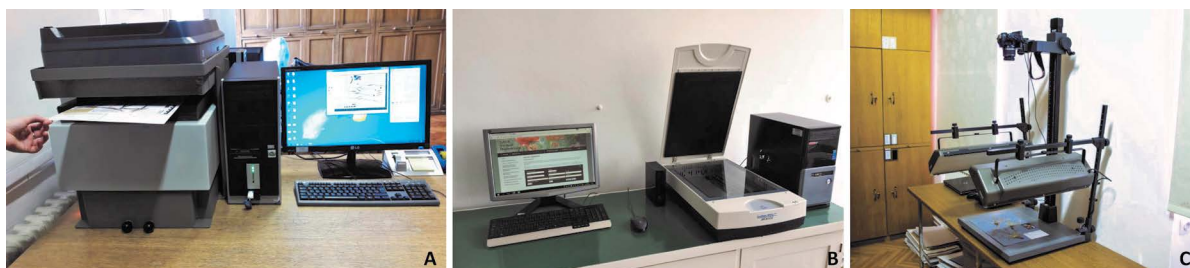
Figure 2. Digitization equipment: a) inversed Epson Expression 11000XL Pro A3 scanner (ZA & ZAHO), b) Microtek ScanMaker 9800 XY Plus scanner (ZAGR), c) DSLR digital camera Canon EOS Digital Rebel XSi 450D with Canon 18 - 55 mm focal length (CNHM).
