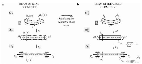
Figure 1 Configurations of the beam example: (a) the observed "real case" problem, and (b) the "ideal case" substitution problem
