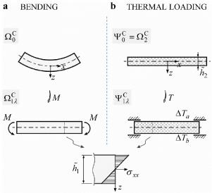
Figure 2 Stress distribution in the beam configuration  $\Omega_{12}^C$ , obtained: a by bending initially curved beam from its stress-free configuration  $\Omega_0^C$ , and b by enforcing thermal dilatation in stress-free configuration  $\Psi_0^C$  of the TM model
