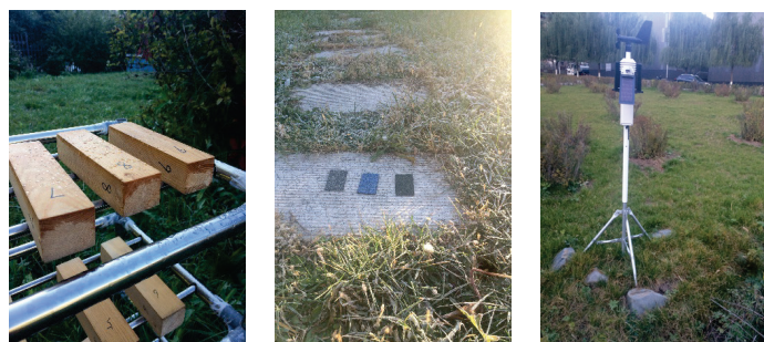
Figure 2 Dew monitors and weather station (Left: poplar wood stick; Middle: asphalt block; Right: weather station)
