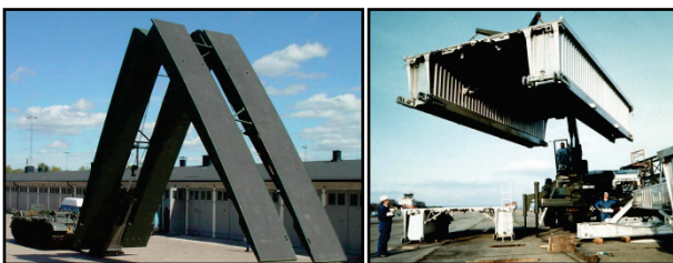
Figure 12 Sweden (left) and German (right) military prefabricated bridges [15]
