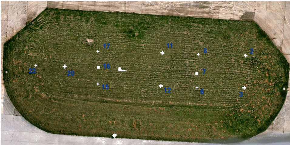
Figure 8. Calibration field at the military airport in Pula (TP-006 2008).
