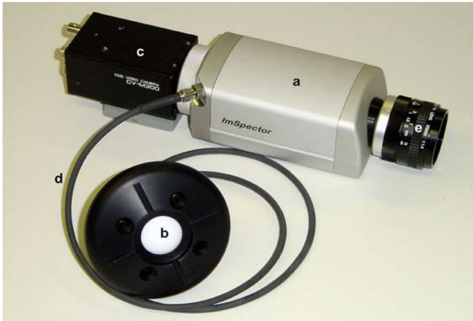
Figure 3. a) Hyperspectral scanner ImSpector V9, b) diffuse light collector – Phodis, c) CCD sensor PixelFly, d) Optical cable, Schneider-Kreuznach lens f = 24 mm (Bajić et al. 2004).
