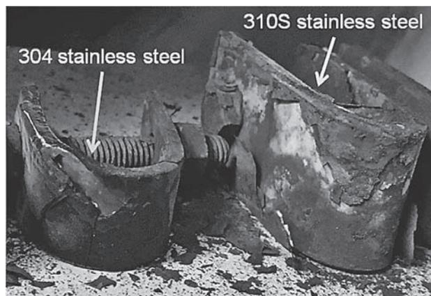
Figure 5 Test specimen after exposed to 210 hrs. 6 mol/l chloride environment at 900 °C
