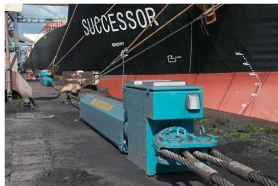
Fig. 12 – Hydraulic mooring system. Source: KRVE (2016)
