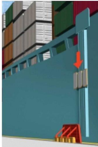
Fig. 13 - Iron Sailor device. Source: Cavotec.
