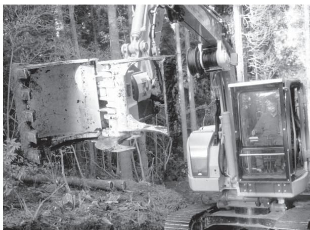
Fig. 24 Excavator with bucket, which can be rotated, and a felling knife
