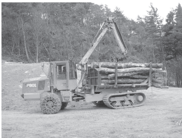
Fig. 15 Articulated forwarder with rubber crawler
