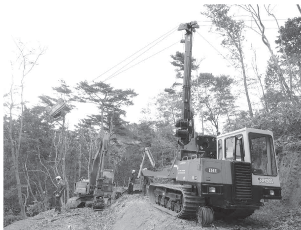
Fig. 2 Interlocked three drums tower yarder which can operate both downhill and uphill
