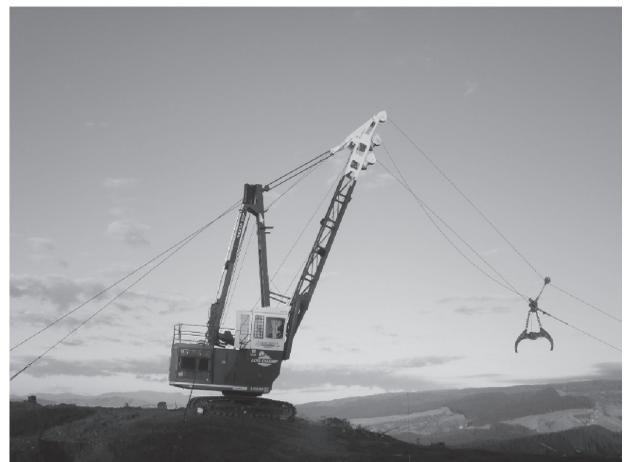
**Fig. 3** T-Mar Log Champ 650 shown above, like Madill 124, is a very large (70+ tonne) swing yarder designed for larger scale mechanised clear-cut operations
