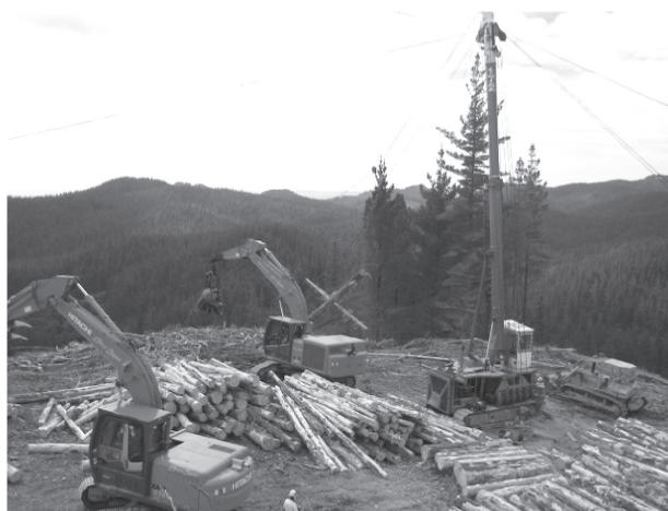
**Fig. 1** A typical PNW or NZ yarder set-up, with a Madill 172 working a larger clear-cut operation from a purpose built landing
