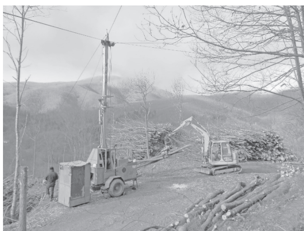
Fig. 4 A light tower yarder routinely used in coppice operation
