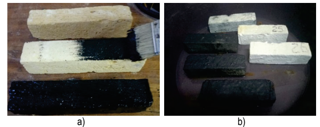
Figure 5 Application of bitumen-rubber and acrylic mastics
