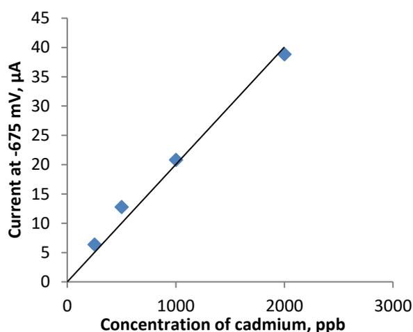
**Fig. 2.** Calibration plot of peak currents at -675 mV against Cd concentration in 0.1 M acetate buffer pH 4.50, containing 80 ppm Hg(NO<sub>3</sub>)<sub>2</sub> and 0.2 M KNO<sub>3</sub>.
