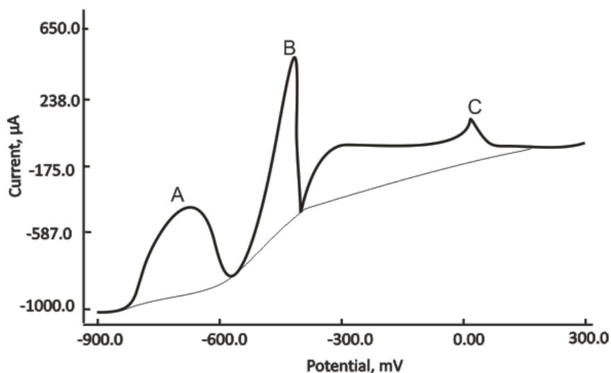
**Fig. 3.** Voltammograms of the soil sample from Abare AB 04 in 0.1 M acetate buffer, pH 4.5 containing 80 ppm  $\text{Hg}(\text{NO}_3)_2$  and 0.2 M  $\text{KNO}_3$ . Peaks A, B and C correspond to Cd, Pb and Cu respectively.
