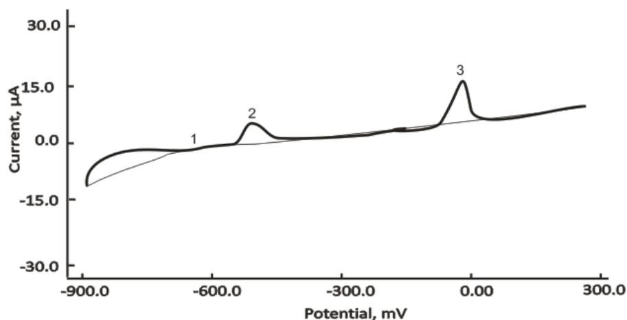
**Fig 5.** Voltammogram of millet leaves from Dareta in 0.1M acetate buffer, pH 4.5, containing 80 ppm  $\text{Hg}(\text{NO}_3)_2$  and 0.2 M  $\text{KNO}_3$ . Peaks 1, 2, and 3 correspond to Cd Pb and Cu
