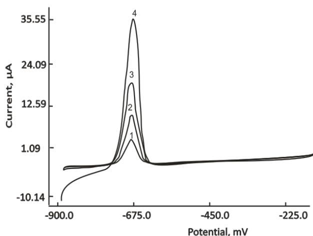
**Fig. 1.** Overlay of the voltammograms obtained for standard solutions of Cd(NO<sub>3</sub>)<sub>2</sub>·4H<sub>2</sub>O in 0.1M acetate buffer, pH 4.5 containing 80 ppm Hg(NO<sub>3</sub>)<sub>2</sub> and 0.2 M KNO<sub>3</sub>. Cd concentration: 250 ppb (1), 500 ppb (2), 1000 ppb (3), 2000 ppb (4).
