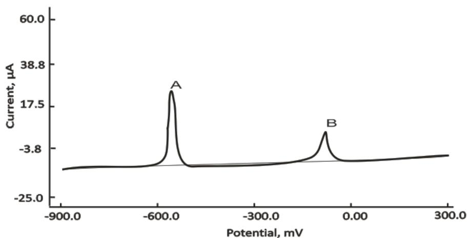
**Fig. 4.** Voltammogram of the soil sample from Abare, AB 13 in 0.1 M acetate buffer, pH 4.5 containing 80 ppm  $\text{Hg}(\text{NO}_3)_2$  and 0.2 M  $\text{KNO}_3$ . Peaks A and B correspond to Pb and Cu, respectively.
