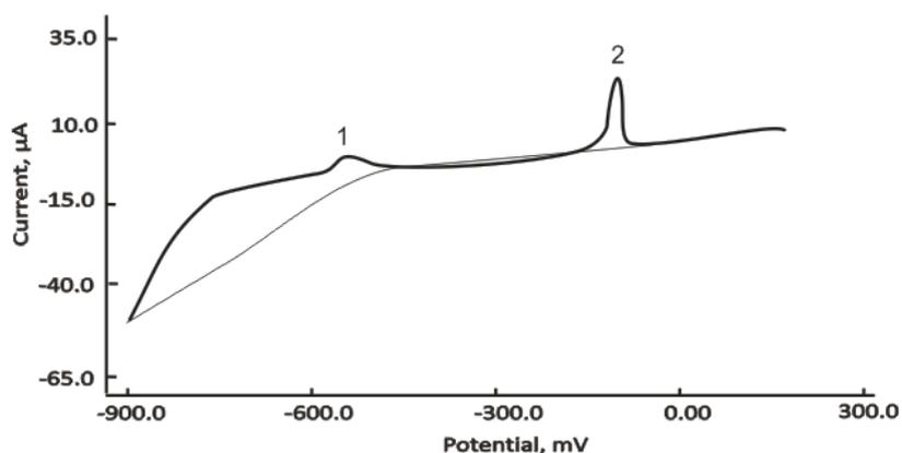
**Fig. 6.** Voltammogram of guinea corn seed from Daretta in 0.1 M acetate buffer pH 4.5, containing 80 ppm  $Hg(NO_3)_2$  and 0.2 M  $KNO_3$ . Peaks 1 and 2 correspond to Pb (-495 mV) and Cu (-19.4 mV)
