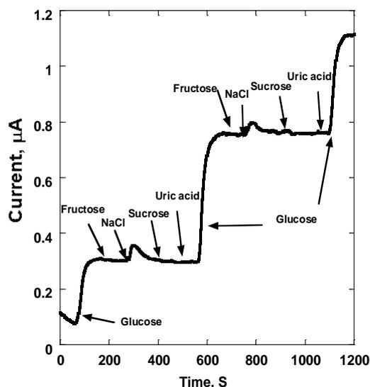
**Figure 10.** Current versus time curve of PG-CNF-(Poly-BiPy-OsCl)-GOX in 50 mM acetate buffer, pH 5.5 at 0.35 V vs. Ag/AgCl after continuous addition of glucose, fructose, sodium chloride sucrose and uric acid
