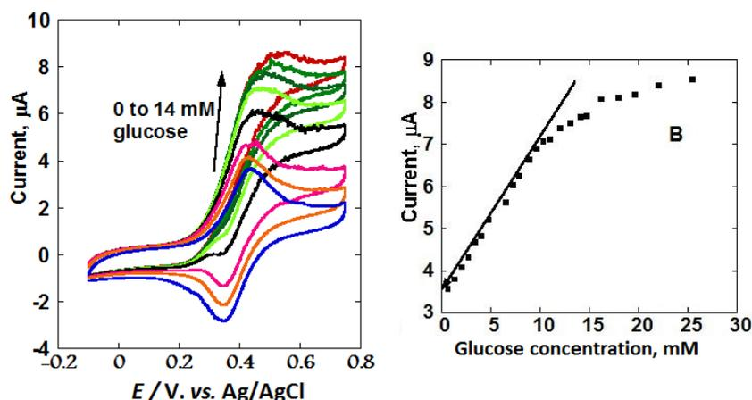
**Figure 6.** (a) Cyclic voltammograms of PG-CNF-(Poly-BiPy-OsCl)-GOX in 50 mM acetate buffer, pH 5.5, recorded at 50 mV s<sup>-1</sup> scan rate after continuous addition of glucose; (b) calibration curve for glucose
