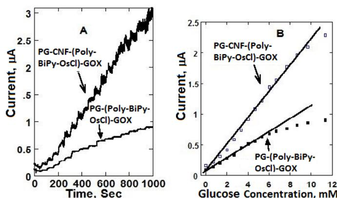
**Figure 8.** (a) Current versus time curve of PG-CNF-(Poly-BiPy-OsCl)-GOX and PG-(Poly-BiPy-OsCl)-GOX in 50 mM acetate buffer, pH 5.5, at 0.35 V vs. Ag/AgCl after continuous addition of glucose (b) Comparison of current versus glucose concentration for PG-(Poly-BiPy-OsCl)-GOX and PG-CNF-(Poly-BiPy-OsCl)-GOX sensors.
