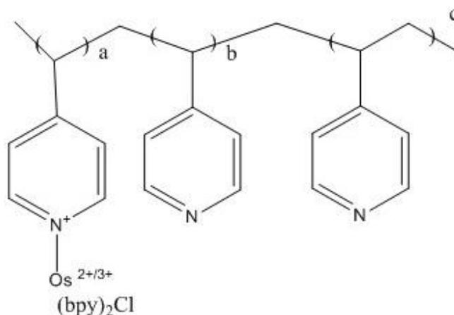
**Figure 1.** Structure of poly[vinylpyridine Os(bipyridine)<sub>2</sub>]Cl redox polymer, (Poly-BiPy-OsCl) ( $a = 1$ ,  $b = 4$ ,  $c = 1$ ) are based on initial reaction conditions
