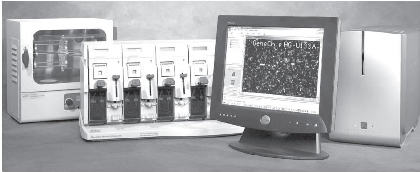
SLIKA 4. Sustav platforme Affymetrixa FIGURE 4. Affymetrix platform system
