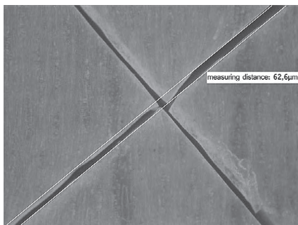
Figure 8 Microscopic image (10x magnification) of a cross-cut of an HW sample with intact coating on its surface. The edges of the cut are smooth and without detachments. 0 % of the cut area is affected by flaking Slika 8. Mikroskopska slika (uvećanje 10 puta) zarezane mrežice HW uzorka s nepropusnim premazom na površini; rubovi rezanja glatki su i bez odvajanja; ljuštenja površine zarezivanja nije bilo
