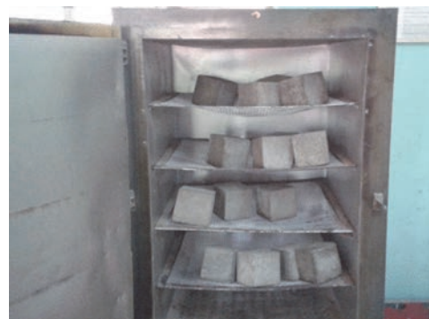
Figure 2. Concrete cubes in oven
