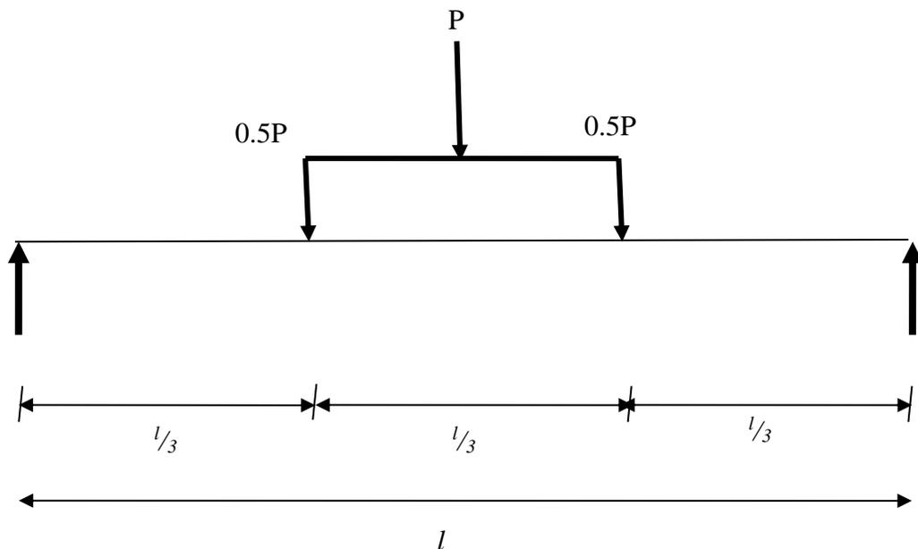
Figure 1. Structural configuration for third point loading.
