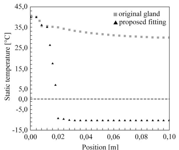
Figure 4. The course of heat distribution from copper pipes to Al-Mg collector casing using the original gland (a) and proposed thermal insulation fitting (b).
