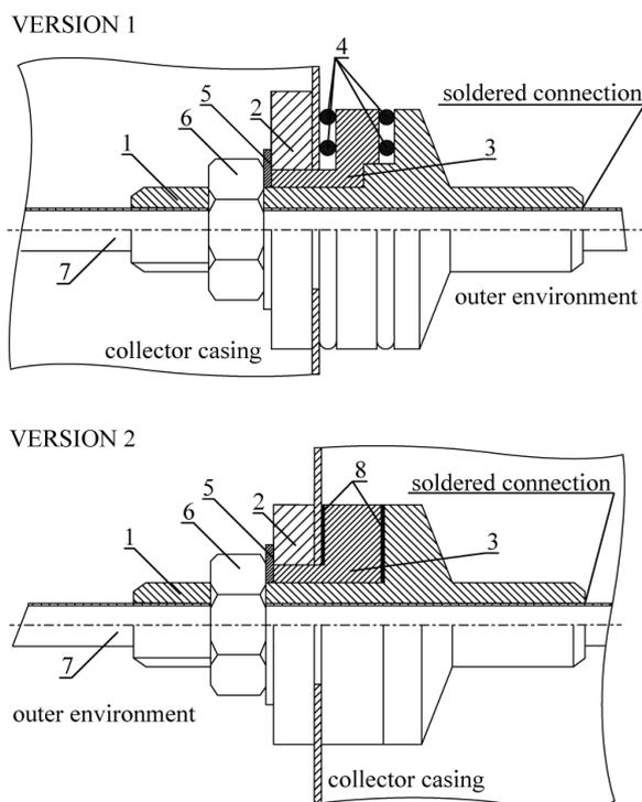
Figure 1. Design of vacuum insulation fitting in two versions - with silicone O-rings, and the layer of sealant.
