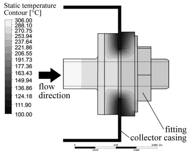
Figure 3. Temperature map in the plane of longitudinal cut in the fitting at the stagnation state of the solar collector.
