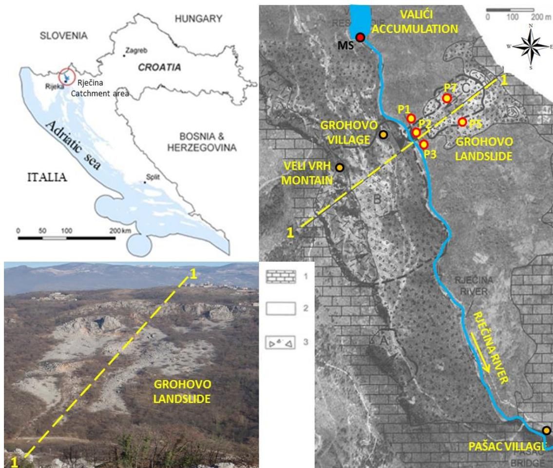
Figure 1. Grohovo landslide location with data sampling points: 1 - carbonate bedrock; 2 - flysch deposits covered by primarily fine-grained slope deposits; 3 - flysch deposits covered by rockfall talus;  $P_i$  - piezometers; MS - meteorological station [17].
