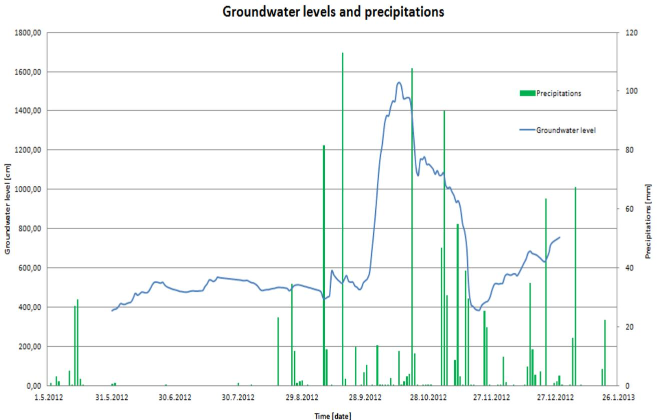
Figure 2. Time series plot of the measured groundwater levels and precipitations (rainfalls).
