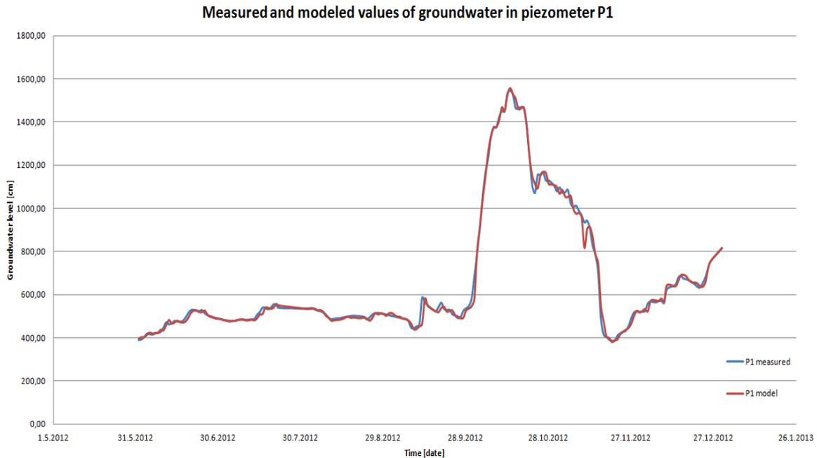
Figure 3. Measured and modeled groundwater level data on piezometer P1-time series for the first model-24 hours prediction.
