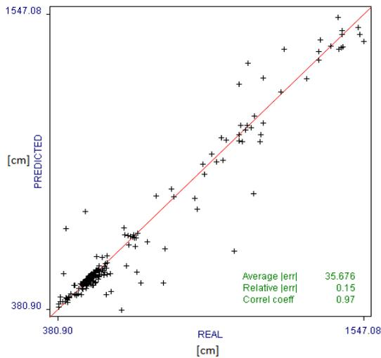
Figure 4. Measured and predicted (modeled) values of groundwater level in cm on piezometer P1 for the second model-48 hours prediction.
