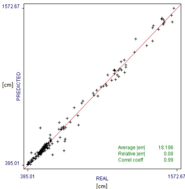
Figure 2. Measured and predicted (modeled) values of groundwater level in cm on piezometer P1 for the first model-24 hours prediction.
