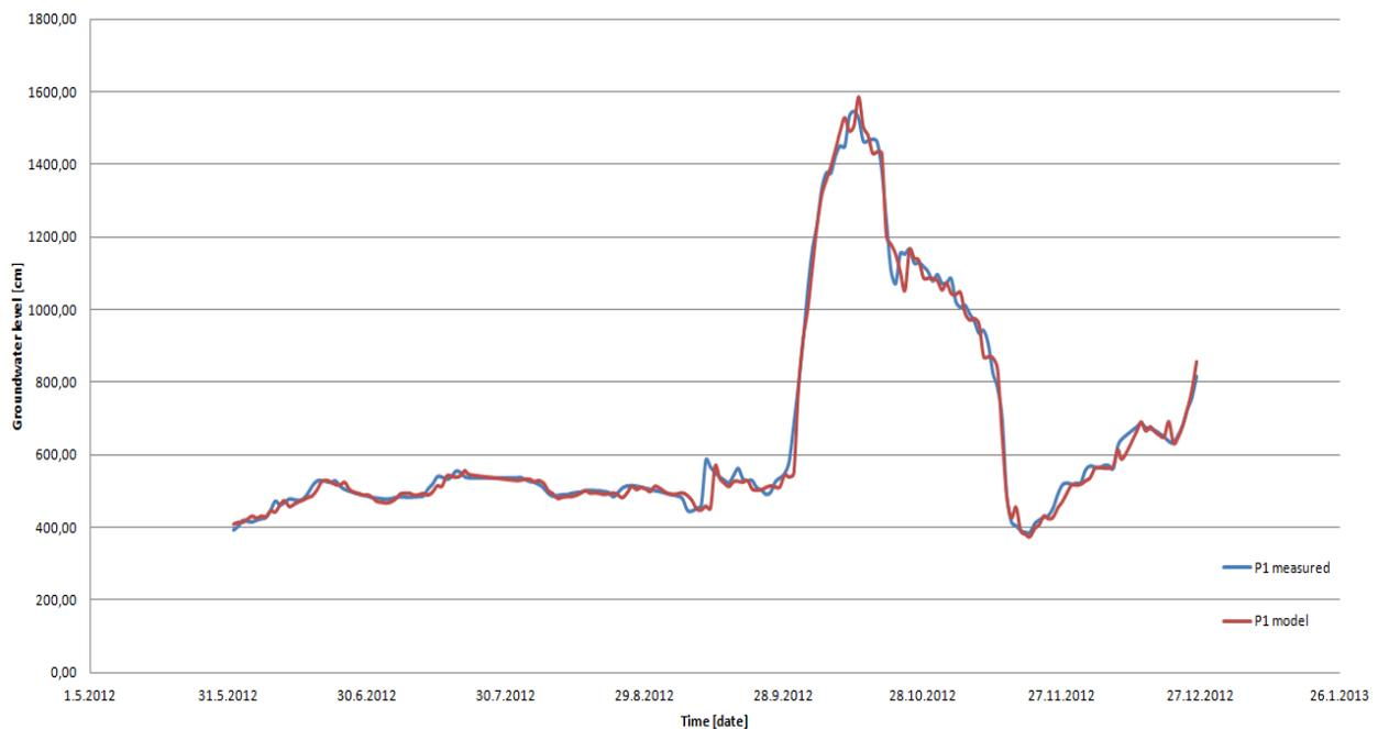
Figure 5. Measured and modeled groundwater level data on piezometer P1-time series for the second model-48 hours prediction.
