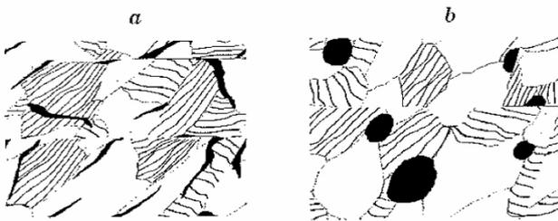
**Figure 1** The microstructure of gray iron (left) and nodular iron (right) [3]
