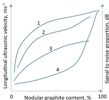
**Figure 2** Longitudinal ultrasonic velocity and signal to noise proportion versus size and content of nodular graphite, [2]
