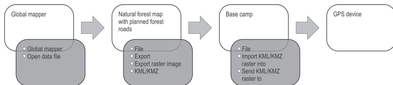
**Fig. 2** Process of sending of planned forest roads into GPS device
