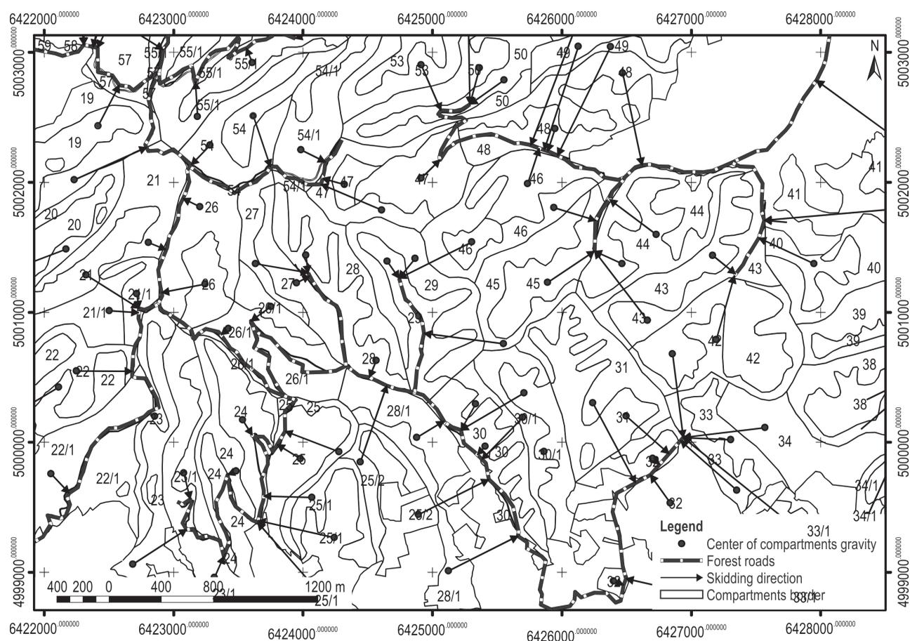
Fig. 3 Determination of average skidding distance
