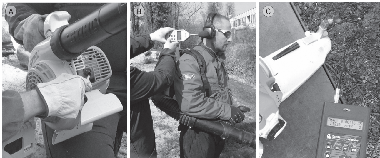
Fig. 1 A) VOC emission measurement on a blower, placing the sensor probe as close as possible to the gas output; B) operator's ear noise measurement; C) detail of the tri-axial accelerometer fixed on the chain saw driving handgrip
