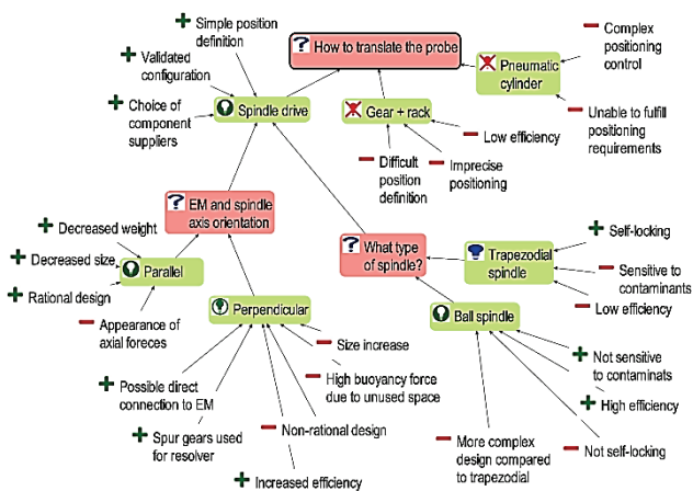
Figure 5 IBIS diagram created using the custom developed tool
