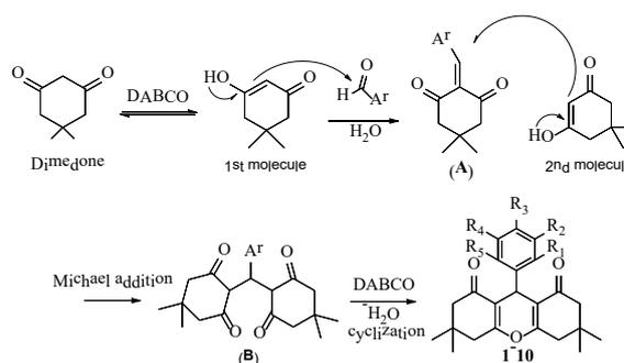
**Figure 1.** Mechanism of synthesis of 2,2,5,5-tetramethyl-9-aryl-3,4,5,6,7,9-hexahydro-1*H*-xanthene-1,8(2*H*)-diones.<sup>[19]</sup>
