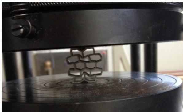
**Fig. 4** Testing the edgewise compression of honeycomb cellular cores
