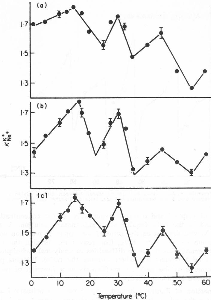
Figure 5. Selectivity coefficient of water in silica gel as function of temperature (top to bottom for  $K^+ - Na^+ - SO_4^{2-}$ ;  $K^+ - Na^+ - I^-$ ;  $K^+ - Na^+ - Cl^-$ ). Data by Wiggins.
