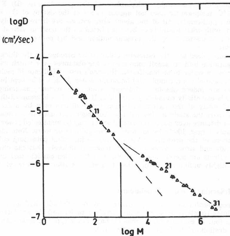
Figure 10.  $\log$  (diffusion constant) as function of  $\log$  (molecular weight). The points represent data for solutes ranging from  $H_2$  (# 1) to hemocyanin (# 31). Data by Stein and Nir.
