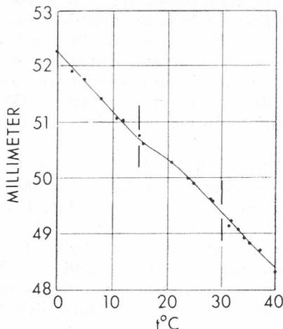
Figure 6. Capillary rise height of water as function of temperature. Capillary diameter 0.585 cm. Data by Brunner (1847).
