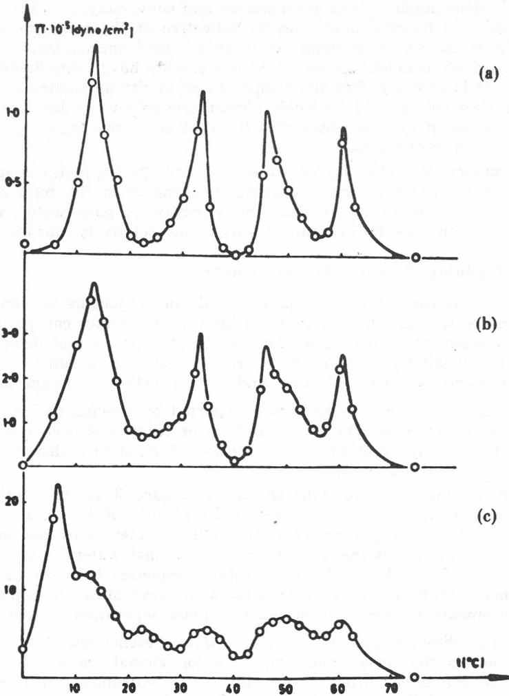
Figure 3. Disjoining pressure of water between quartz plates as function of temperature for three plate separations (top to bottom: 0.05; 0.03 and 0.01  $\mu\text{m}$ ). Data by Peschel and Adlfinger.
