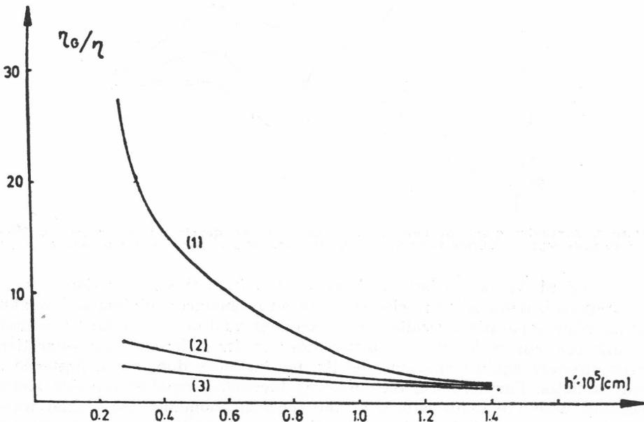
Figure 1. Relative viscosity of water at  $20^\circ\text{C}$  between quartz plates as a function of plate separation. Data for three values of applied force: (1)  $F = 253$ ; (2)  $F = 523$  and (3)  $F = 657$  dynes. Data by Peschel and Adlfinger.
