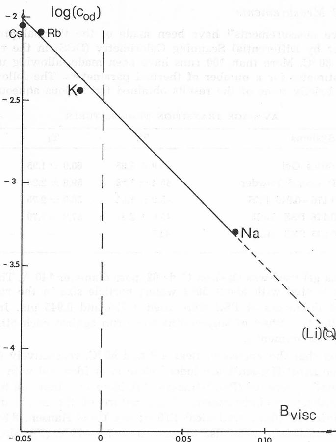
Figure 9.  $\log$  (concentration of onset of deviation) as function of viscosity  $B$ -coefficient for Cs, Rb, K, and Na Chloride. Value for LiCl by extrapolation.
