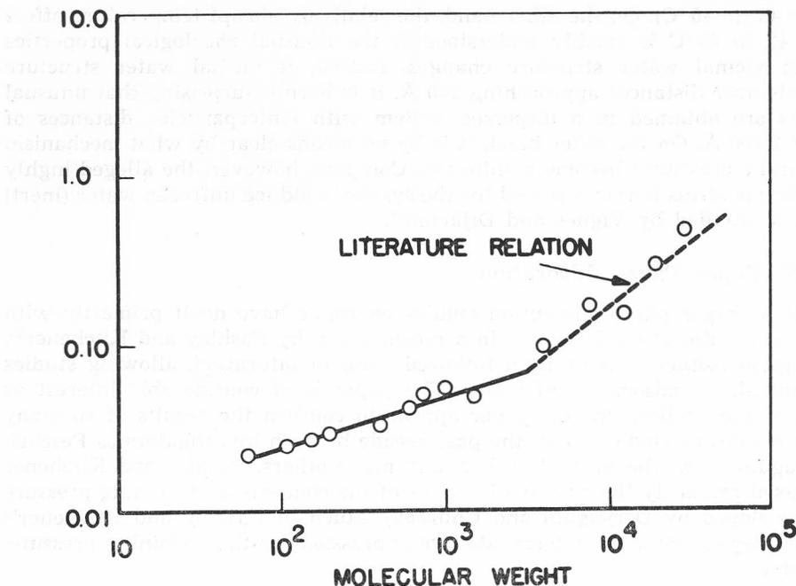
Figure 11. Intrinsic viscosity of polyethylene oxide in water (at 30 °C) as function of molecular weight. Data by Schick, quoted by Bailey and Koleske.
