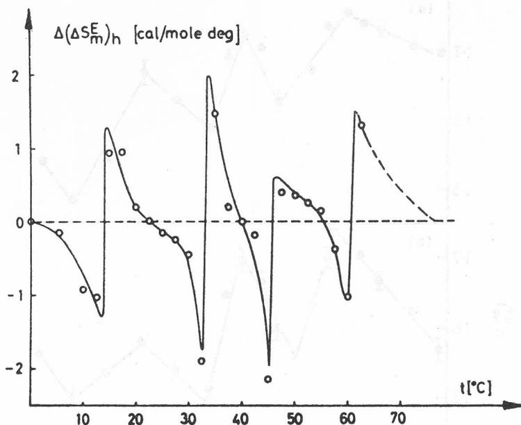
Figure 4. Differential molar excess entropy of water between quartz plates as function of temperature. Plate separation  $0.05 \mu\text{m}$ . Data by Peschel and Adlfinger.
