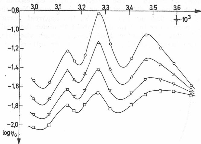
Figure 2. Arrhenius graph of viscosity of water between quartz plates for four different average plate separations (top to bottom: 0.03; 0.05; 0.07; 0.09  $\mu\text{m}$ .) Data by Peschel and Adlfinger.
