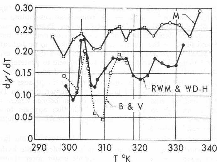
Figure 7. Numerically differentiated surface tension data for water as function of temperature.
