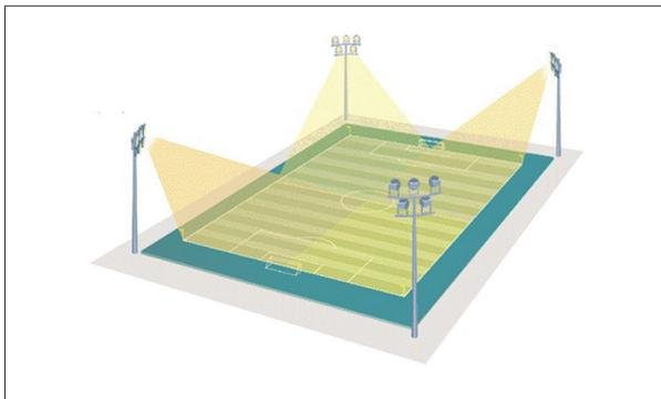
Figure 4 Four Lighting Tower Arrangement [2]
