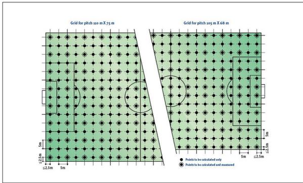
Figure 3 Calculation Grid Points [2]
