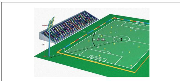
Figure 5 Minimum Lighting Tower Height [2]
