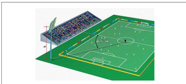
Figure 5 Minimum Lighting Tower Height [2]
