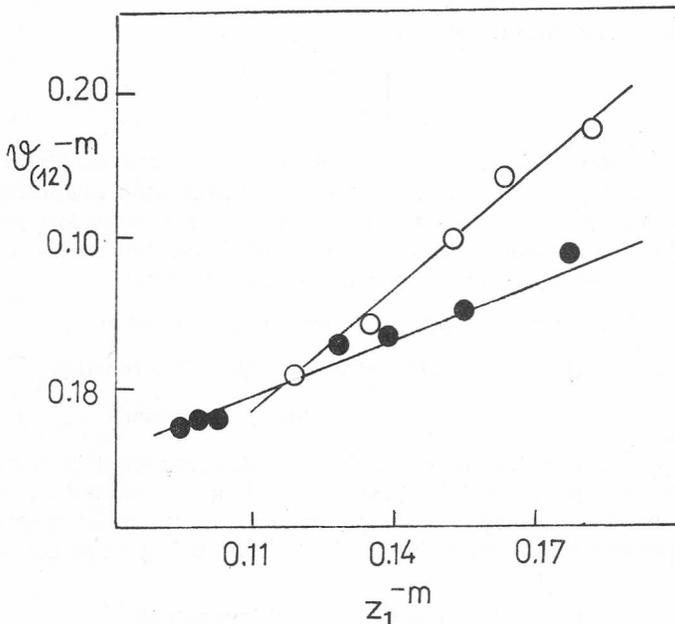
Figure 2. Linear dependences  $N_{(1,2)}^{-m}$  vs  $z_1^{-m}$  for adsorption isotherms (27): (●) C<sub>3</sub>H<sub>8</sub>-C<sub>2</sub>H<sub>6</sub> at 293 K, (O) C<sub>3</sub>H<sub>6</sub>-C<sub>2</sub>H<sub>4</sub> at 293 K on charcoal »Nuxit-Al«.  $r_{21}$  has been calculated from eq. (29b).
