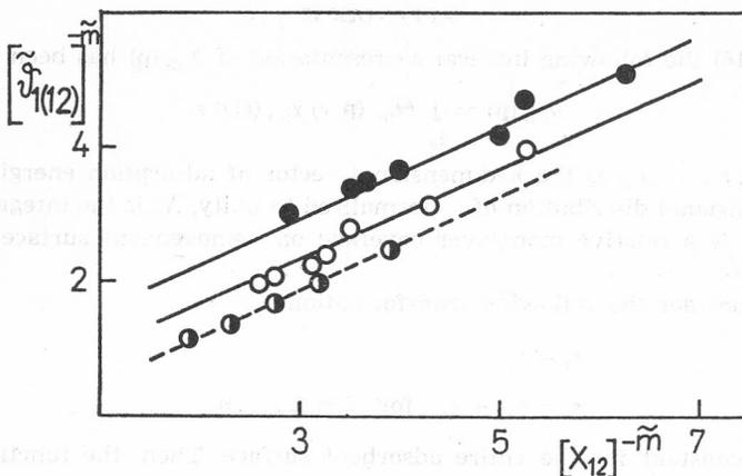
Figure 3. Linear dependences  $\tilde{v}_{1(12)}^{-\tilde{m}}$  vs.  $x_{12}^{-\tilde{m}}$  for binary liquid mixtures on aerosil: (1) benzene-(2)isooctane at 303 K (dashed line):  $m = 0.45$ , and (1) benzene-(2)CCl<sub>4</sub> at 303 K (solid line -○);  $m = 0.45$ , and 338 K (solid line -●);  $m = 0.50$ .
