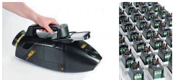
Figure 6. a) The VASOR136 contains b) 36 cartridges each containing one bee. [26]: “Filtered in by a standard gas mask cartridge is a constant supply of clean air. When an operator presses a button on the VASOR, an air sample is taken from the environment that exposes the bees to ambient, unfiltered air. If the bees have been trained to respond to a vapor in that air, the bees will exhibit a proboscis extension reflex response and the response will be translated by the VASOR into a simple result shown on the screen display”.
