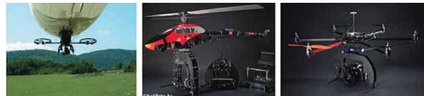
Figure 5. The unmanned aerial vehicles (UAV) with electric engines, available in Croatia for the considered purpose. All are radio controlled and provide route on the digital moving map. a) Blimp, payload 1 kg, endurance 1 h. b) UAV helicopter, endurance 10 min. c) Hexacopter, endurance 20 min.
