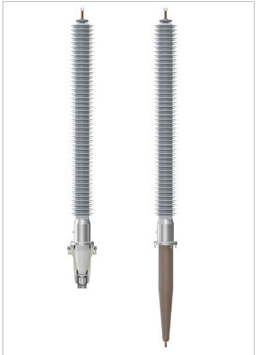
Figure 9. Length comparison showing a conventional bushing alongside a pluggable bushing. With the pluggable bushing, the installation depth in the transformer is reduced by about a third. (Example for 245 kV: pluggable system 470 mm inside transformer, conventional 620 mm [1])
