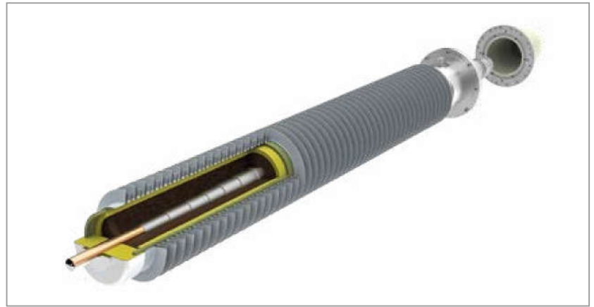
Figure 2. Composition of a pluggable HV-CONNEX Gr. 7-S bushing up to 362 kV. Heat pipe technology for cooling the conductor enables maximum currents in a minimum of space
