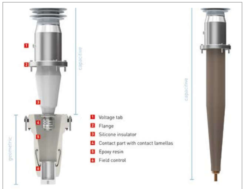
Figure 3. Contact and flange region of a pluggable bushing
