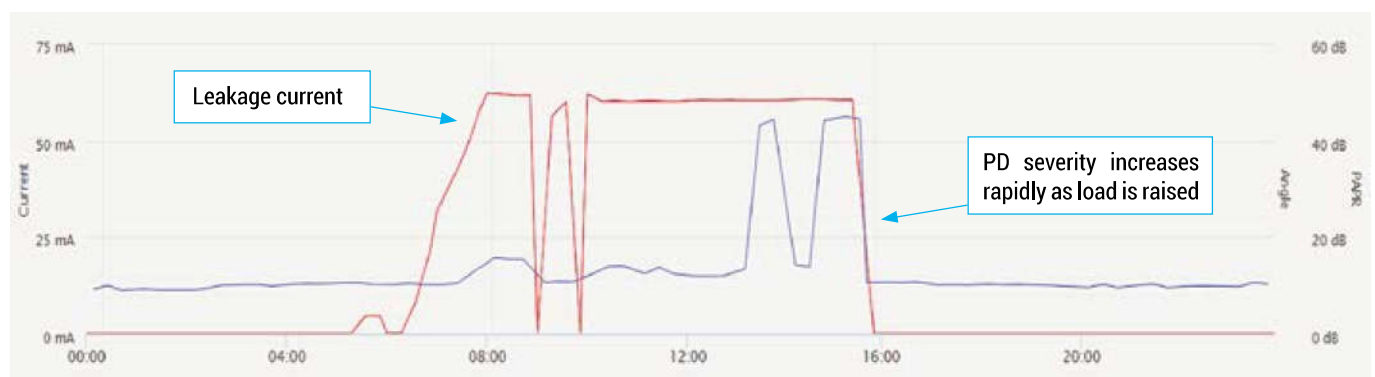
Figure 5. Bushing leakage current and PD levels on energization of a GSU transformer
